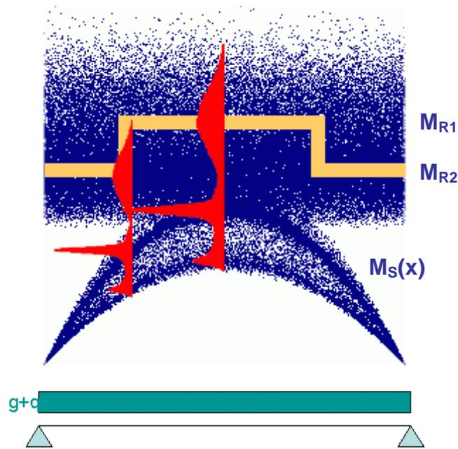
Fig. 13 Response and resistance, bending moments  $M_S$ ,  $M_{R1}$ ,  $M_{R2}$
